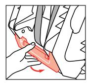
You may need to remove the base for narrow vehicle seats or airline use. See "Removing Base" in Belt-Positioning Booster section. To use the child restraint rear-facing without base, make sure recline stand is folded under seat.
